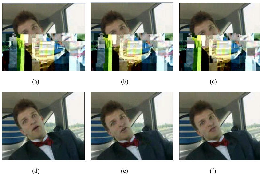
FIGURE 8. Triplets of sample frames of the received decoded sequence (single-user transmission, SNR of the FGST layer = 10dB): (a), (b), (c): single-layer MC-SS transmission, (d), (e), (f): VBR MC-SS transmission with multi-layered coding
