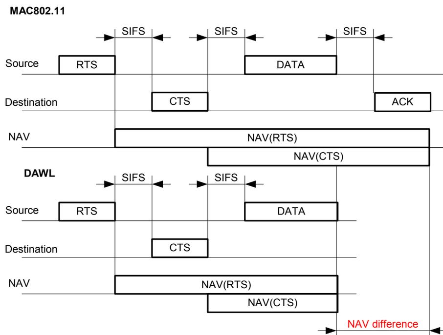
**Figure 3.** The difference between NAV calculation in the original 802.11 and DAWL protocols.
