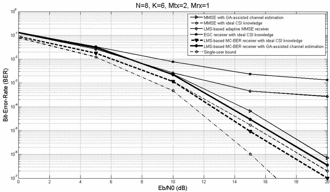
**Figure 5.** BER performance yielded by the LMS-based MCBER (with ideal CSI knowledge and GA-assisted channel estimation), EGC (with ideal CSI knowledge), LMS-based MMSE and ideal MMSE (with ideal CSI knowledge and GA-assisted channel estimation) multi-user detectors for  $N=8$  subcarriers and  $K=6$  users
