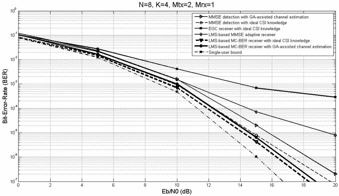
**Figure 4.** BER performance yielded by the LMS-based MCBER (with ideal CSI knowledge and GA-assisted channel estimation), EGC (with ideal CSI knowledge), LMS-based MMSE and ideal MMSE (with ideal CSI knowledge and GA-assisted channel estimation) multi-user detectors for  $N=8$  subcarriers and  $K=4$  users
