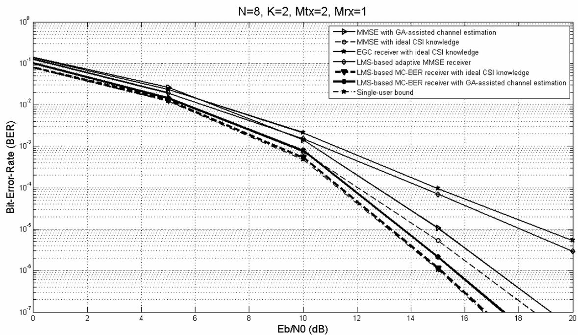
**Figure 3.** BER performance yielded by the LMS-based MCBER (with ideal CSI knowledge and GA-assisted channel estimation), EGC (with ideal CSI knowledge), LMS-based MMSE and ideal MMSE (with ideal CSI knowledge and GA-assisted channel estimation) multi-user detectors for  $N=8$  subcarriers and  $K=2$  users
