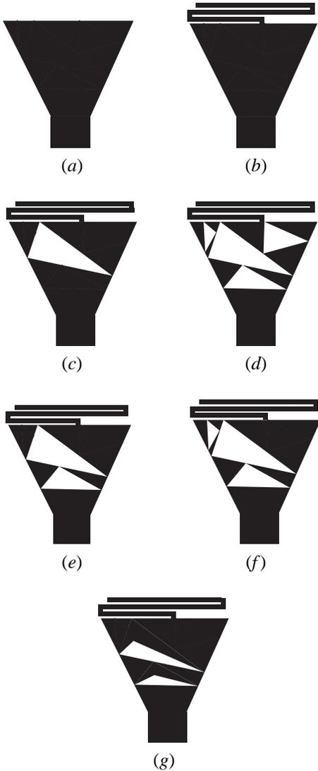
Fig. 4. Three-band hybrid prefractal antenna - Intermediate geometries.
