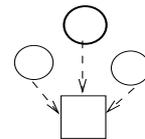
Fig. 2. Example of distributed access control: the squared node obtains the required authorization to join the network of Figure 1 from at least three nodes of middle or lower level, among which at least one of middle level.
