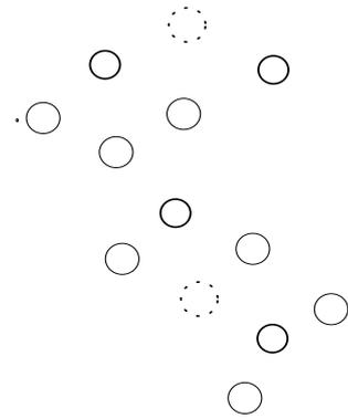
Fig. 1. Example of hierarchical WSN structure: dashed line nodes consist on nodes of higher level; thick solid line nodes are middle level nodes; thin solid line nodes consist on nodes of lower level.
